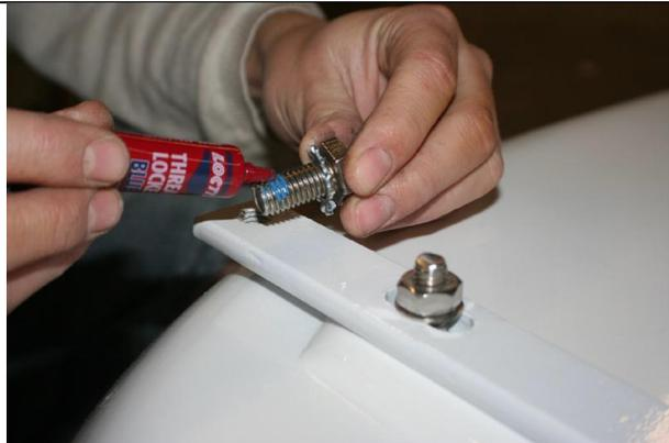
6. Tighten the claw foot fixing bolt; make sure it fits well against the tub. If the foot doesn't fit well, adjust by sliding the holding bar. When everything fits well, tighten the nuts fully to studs on the tub.
